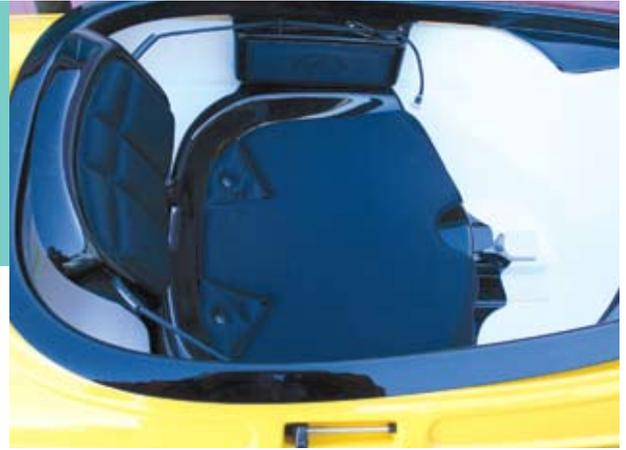
The seat can be adjusted forward and aft for comfort and boat trim.
